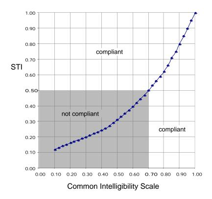
The appendix of NFPA 72 calls for a minimum intelligibility of 0.70 on the CIS scale, which corresponds to an STI of 0.50. A voice alarm system performing at or above either
